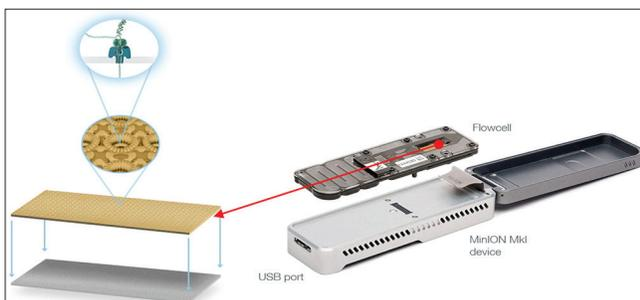
**Figure 1: Miniature nanopore sequencing device with microscopic view of flowcell containing embedded nanopore<sup>[43]</sup>**
