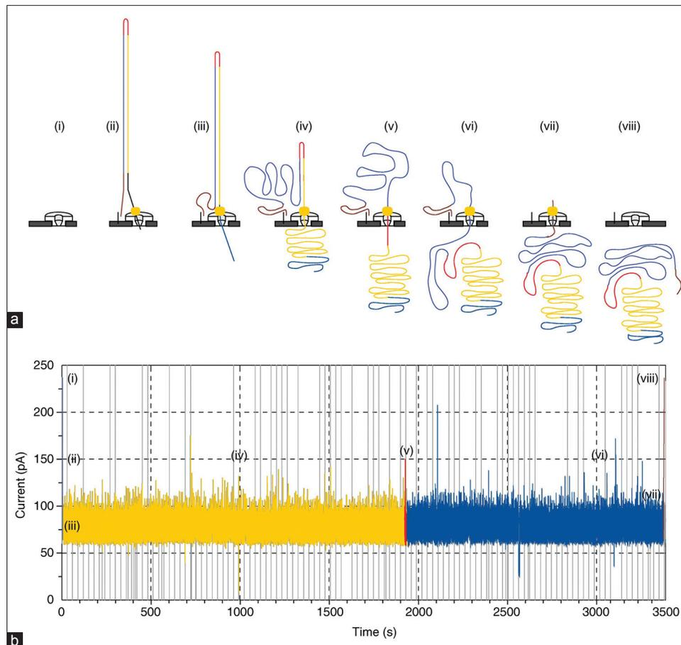
**Figure 2: Principle of nanopore sequencing. (a) Visualization of 2 ssDNA strands connected by adaptor passing through the nanopore. (b) Graphical representation of raw data produced by MinION, also known as "squiggle plot"<sup>[29]</sup>**
